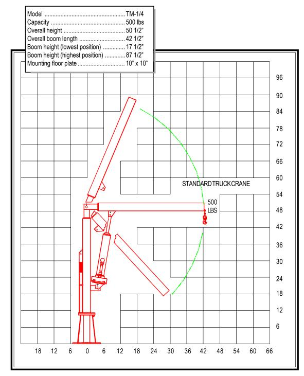
PUMPING CYCLES needed to raise boom through full travel: 90.
