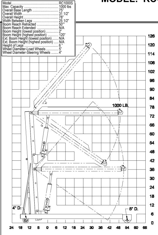
NOTE: Ruger can modify any standard dimensions to meet specific customer needs.
