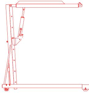
Maximum Value and Safety at a Modest Investment. The RC1000S boom reaches 40" out from ram connecting point and lifts 1000 pounds. Tested and exceeds ANSI/ASME PALD standards. Meets ANSI Z.535
