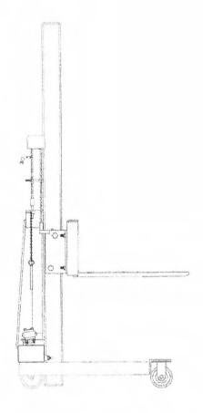
The 10STH comes complete with built-in hydraulics and a needle type release valve for pin-point control. The double acting hand pump simplifies the raising and lowering of loads.
